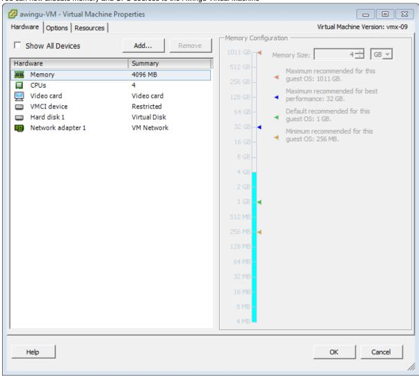
Awingu recommends the following specs for your virtual machine. Those specs are based on carefully performed internal load tests.
