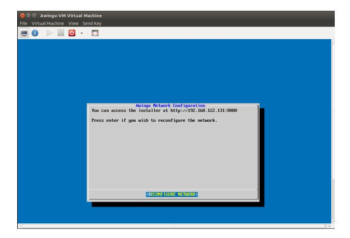
10. After you have configured the network settings for your virtual machine, you can now proceed with the installation through a graphical installer interface. If you need to change your network settings in the future, you can update these here again (not supported for multi node configuration).
