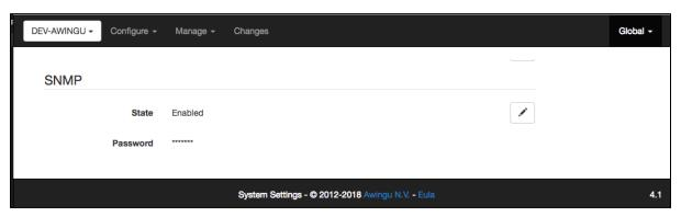
The status and health of Awingu appliances can be monitored and integrated in your monitoring system using SNMP. If enabled, all Awingu appliances provide an SNMP agent which is accessible using SNMPv3.
