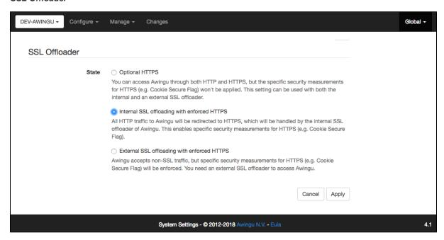
If no external SSL offloader is available, Awingu can handle the SSL offloading (also referred to as SSL termination) internally.
