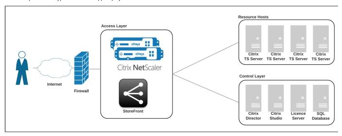
Installing Awingu next to this setup can be achieved by deploying 1 (or more for load distribution or High Availability) Awingu appliance in the Access Layer following this procedure which can be executed in less than 1 hour.
