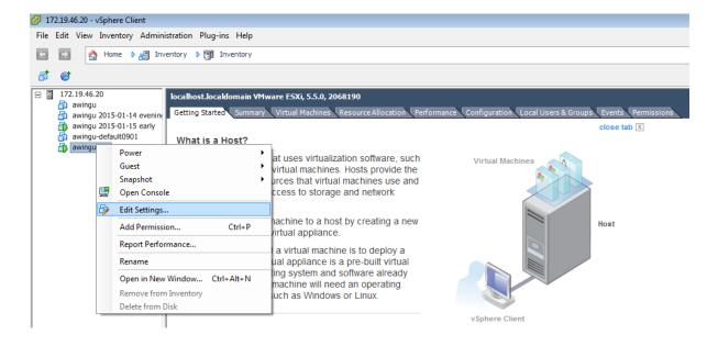
2. You can now allocate memory and CPU sources to the Awingu Virtual Machine
