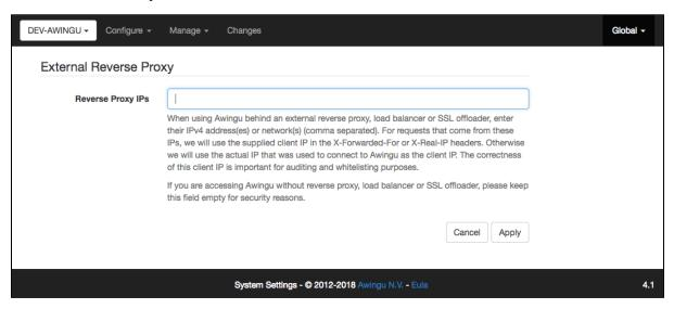
Relevant when using Awingu behind an external reverse proxy, load balancer or SSL offloader. Here you specify their IPv4 address(es) or network(s) (comma separated). For requests that come from these IPs, we will use the supplied client IP in the X-Forwarded-For or X-Real-IP headers. Otherwise we will use the actual IP that was used to connect to Awingu as the client IP. The correctness of this client IP is important for auditing and whitelisting purposes.
