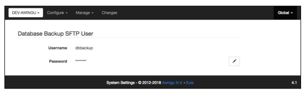
This parameter is only relevant when the Awingu internal database is used. Awingu saves the database to local disk every day. You can retrieve this dump and saving it on another system via SFTP. The dumps are retained on local disk for a period of 3 days, before being discarded. More information: Backup and recovery of the Awingu Database.
