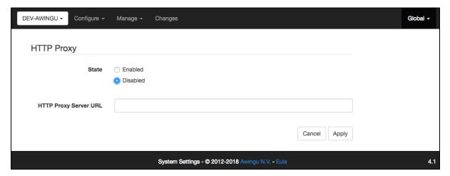
The HTTP Forward Proxy server is configured during the installation and can be edited here. The proxy server will be used to reach public services, like the Repo Server of previous section, DUO MFA, Skype for Business and OneDrive. Note that automatic SSL (Let's Encrypt) is not using this proxy. Please refer to Connectivity Requirements for more details about outbound connections.
