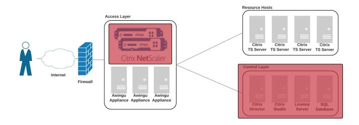
Please note that the Netscaler can be optionally used to loadbalance to the different Awingu appliances but any loadbalancer will do.
