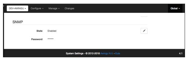
The status and health of Awingu appliances can be monitored and integrated in your monitoring system using SNMP.
