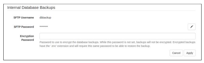
This parameter is only relevant when the Awingu internal database is used. Awingu creates a backup of the internal database every day and store it on the appliance. You can retrieve this backup and save it on another system via SFTP. The backups are retained on local disk for a period of 3 days, before being discarded. More information: Backup and recovery of the Awingu Database.
