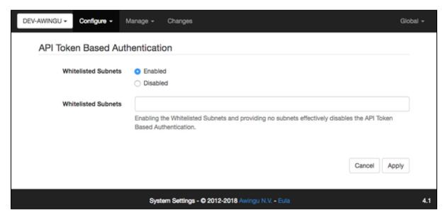
Next to basic authentication with username and password, administrators can use authentication with an API token. This is useful for automation of Awingu through scripts using the REST API. As this token never expires, it is recommended to limit the usage of the token to the network of the computers/servers where the scripts are running using Whitelisted Subnets.
