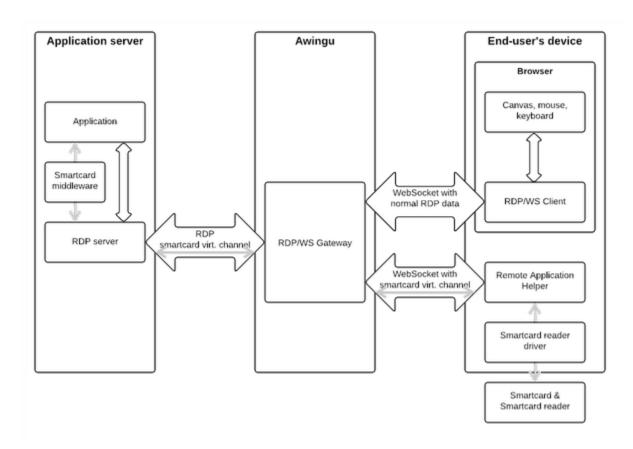
In order to use a smart card in a streamed application, the administrator should explicitly enable smart card support for the application and the user should dispose of a smart card reader connected to his device. When the user launches such a smart card support enabled application, the Awingu portal will connect to the locally installed Remote Application Helper, which will connect to the smart card reader and act as a bridge between the smart card reader and the Awingu portal.
